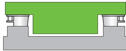
Vibration isolation concrete block or steel platform
