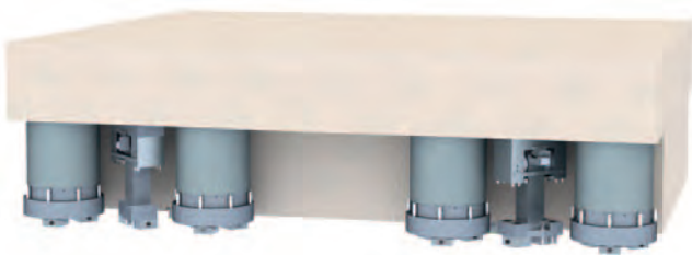
Active vibration isolation AIS™ High Performance by Bilz, which suspends the glass fiber reinforced plastic armoured foundation block weighing 75 tons on air cushions.
